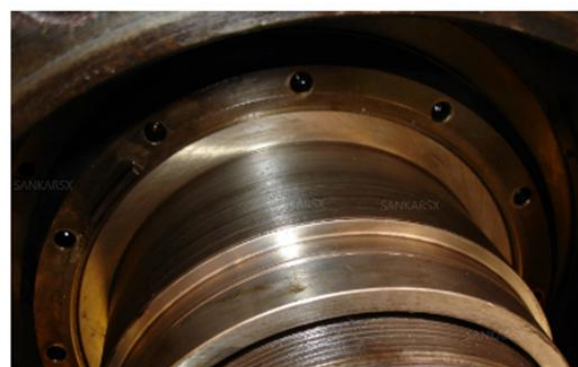
Fig. 8. Cone Seal Abrasion.
