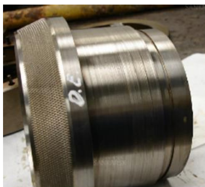
Fig. 6. Drive End Cone Seal Abrasion.
