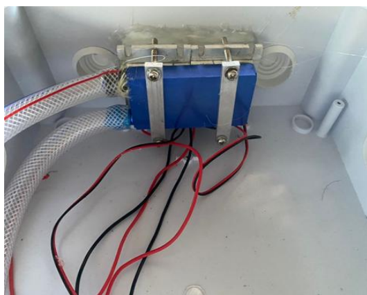
Fig. 1. Thermoelectric Peltier heating unit integrated into the water-heating test rig.
