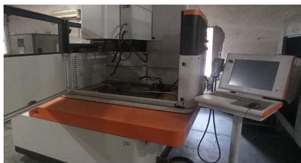
Fig. 1. Pictorial view of EDM Machine used during experimentation.
