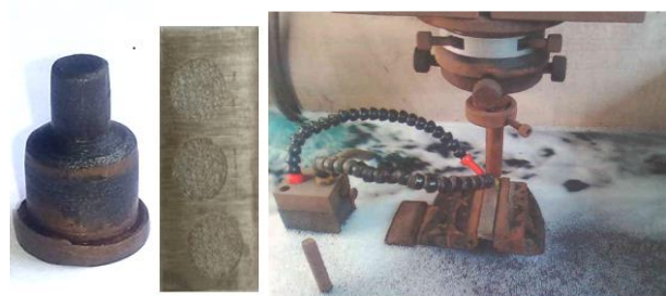
Fig. 2. Pictorial view of Cu electrode, workpiece and experimental Set-up.
