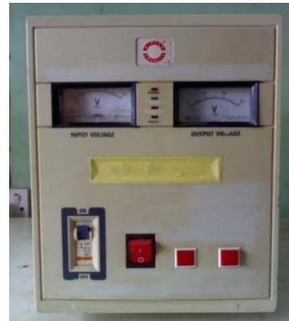
Fig. 9. Front view of the Inverter.
