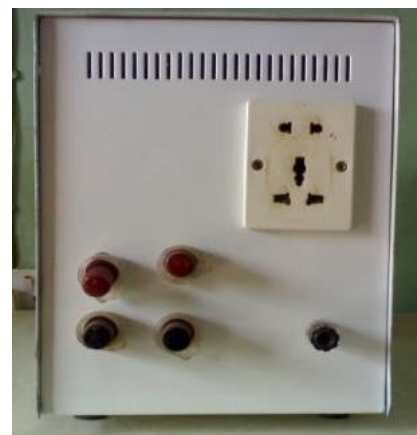
Fig. 10. Back view of an Inverter.
