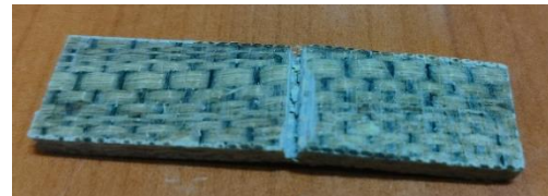
Fig. 11. Impact tested specimen.
