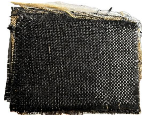
Fig. 5. Composite Material after Demolding.
